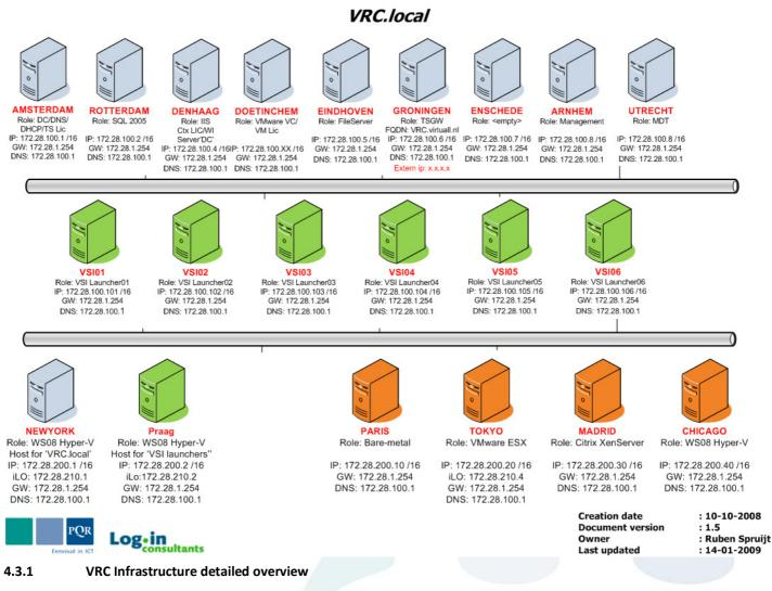
The VRC infrastructure has been designed and implemented to run multiple tests on the four (Bare metal, Hyper-V, XenServer & VMware), different platforms simultaneously. This was essential, as over 150 VSI test-runs have been performed in total.
